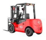
The X5 Series is ideal for medium to heavy-duty operations, from manufacturing and construction to logistics centers and outdoor yards. Its pneumatic tires, 150 mm ground clearance, and sealed electrical components enable smooth, safe operation even on uneven or unpaved surfaces. The modular Li-ion battery system allows companies to expand energy capacity from 280Ah to 560Ah, adapting to single-shift, multi-shift, or seasonal high-demand applications without changing the truck setup.
