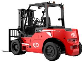
Perfect for steel mills, ports, and heavy-logistics terminals, the EFL703 handles extreme loads with confidence and stability. Its dual-motor PMSM drive, reinforced mast, and rugged chassis ensure reliability in high-load, long-distance, or outdoor operations. Designed for productivity and safety, it provides smooth control and low noise for both operator and environment.
