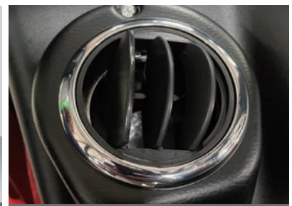
Dashboard with orientable heater outlet
